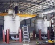
MS Towers, Drums(SA516 G70, SUS304) Towers, Drums, and Etc. were manufactured.
